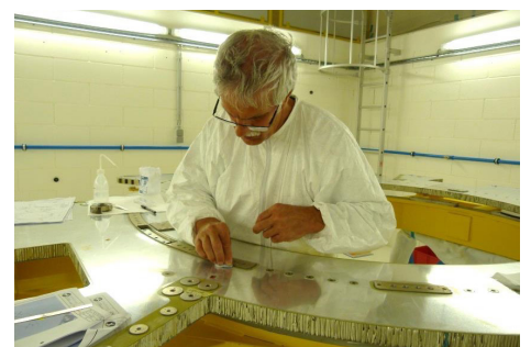
Strain gauging on CSO satellite
